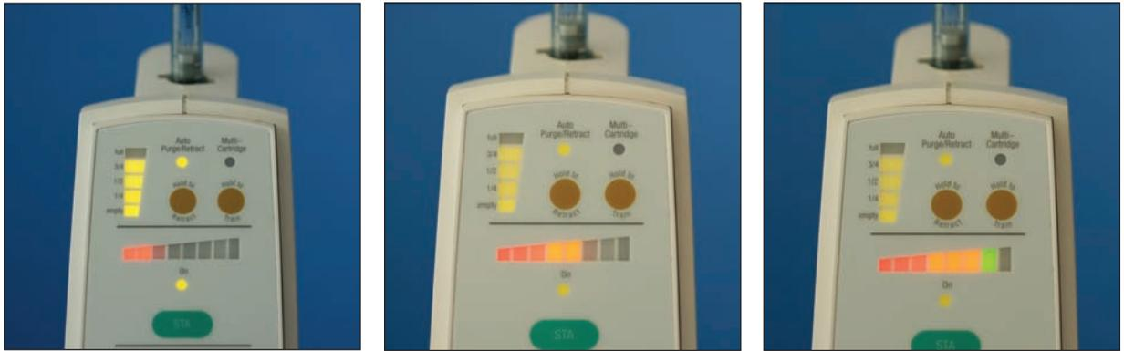
**Figures 3A - 3C**—The STA-System real-time feedback is an audible and a visual pressure sensing scale. The visual scale is displayed on the front panel, composed of a series of LED lights—orange, yellow, and green. The orange lights indicate minimal pressure (Figure 3A), the yellow indicate mild to moderate pressure (Figure 3B), and the green indicate moderate pressure (Figure 3C), indicative of the PDL tissue.
